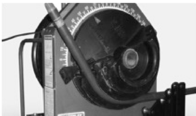
Figure 19: Bender with special shoes required for bending PVC-coated conduit.
