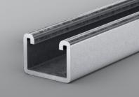
Wheatland Tube's ZI-Strut is made with cold-roll-formed, structural grade carbon steel and engineered with half-slot construction. ZI-Strut is interchangeable with industry-standard 1<sup>5</sup>/<sub>8</sub>" channel profiles.
