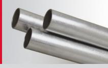
Wheatland Tube's steel EMT is a lightweight wiring solution tough enough for any environment. Our steel EMT is produced from mild steel strip in our state-of-the-art ERW mills using the industry's leading in-line galvanizing process. It is easy to bend, and the proprietary ID coating allows for faster wire-pulling. Wheatland Tube's steel EMT is available in trade sizes ½-4 in eight vivid colors and 10' and 20' lengths.
