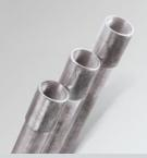
Wheatland Tube's steel intermediate metal conduit provides exceptional physical protection for cables and connectors, including installations in hazardous locations. IMC contains 33% less steel than conventional rigid metal conduit, leading to a lighter weight and a larger inside diameter for faster wire pulling. Wheatland Tube's IMC is available in trade sizes ½-4.
