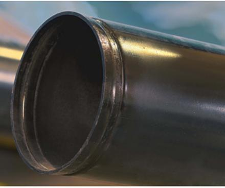
Wheatland's Mega-Flow is an engineered, light-wall steel sprinkler pipe that offers ID up to 7% larger than Schedule 10 and 11% larger than Schedule 40 for improved hydraulics. With its proprietary mill coating, Mega-Flow is an excellent alternative to standard wall products so you can downsize your entire sprinkler system with the same or greater quality.
