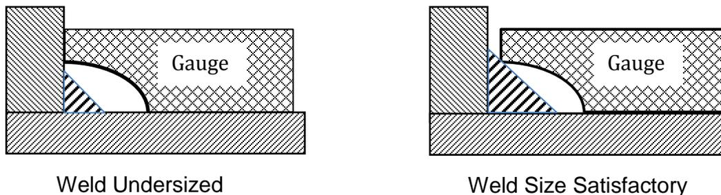
The gauge must touch weld metal before touching the base metal. Where it is difficult to actually measure the entire weld due to the geometry of the members, measure the weld at where it can be measured, then visually check that it is the same width all around. Where the drawing specifies welding all around a joint, the weld size should meet minimum drawing requirements all around the joint.
